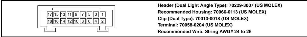
Figure 2-26 DBV-301 ID-002/ID-042/ID-044 Communication Interface Connector Pin Assignment
