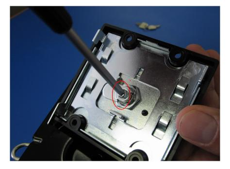
Screw the assembly back on (Reference Assembly) and tighten down the screw.
