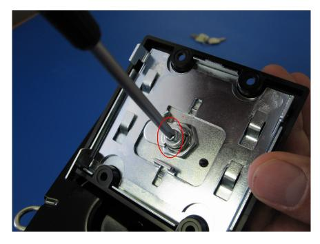
Tighten the nut with socket tool
