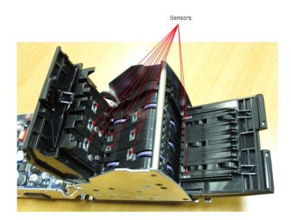
Be sure there is no dust accumulation, scratches or other mechanical damage. Performance will be greatly impacted.
