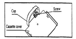
Assemble the cassette cover and the cap with the lock as shown at the picture. Pay your attention on the orientation of the lock and its cam.
