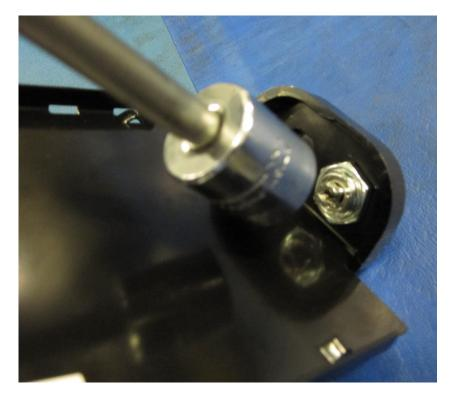
Screw the assembly back (Reference Assembly) on and tighten down the screw.
