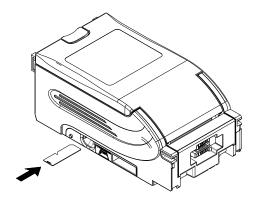
Memory Stick Label should face down and notch on memory stick should face the left as per diagram above.
