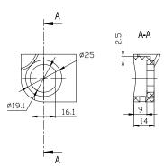
**Detailed Dimension of Slot for Lock**
