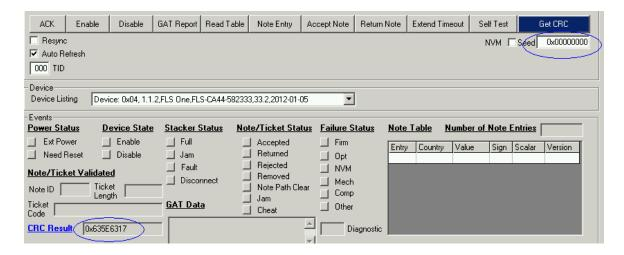
Alternatively, CRC can also be verified by CashCode CRC Verifier or CFS Downloader PC application. Make sure to setup seed 0. Connect PC to USB frontal port of Bill Validator, run the application CRC Verifier and select type of CRC, finally just select **Get CRC**. For more detail refer to Downloader CFS Manual.
