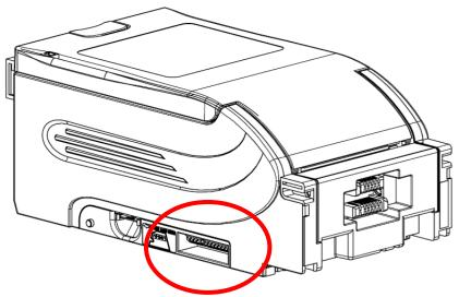
The first series of four (4) DIP switches is defined below. Only the switch 2.4 should be used during operation and diagnostic of the one™ Bill Validator, to switch between:
