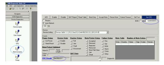
Click on Note Acceptor. Press Disable. Now we ready for self test, press Self Test tab,
