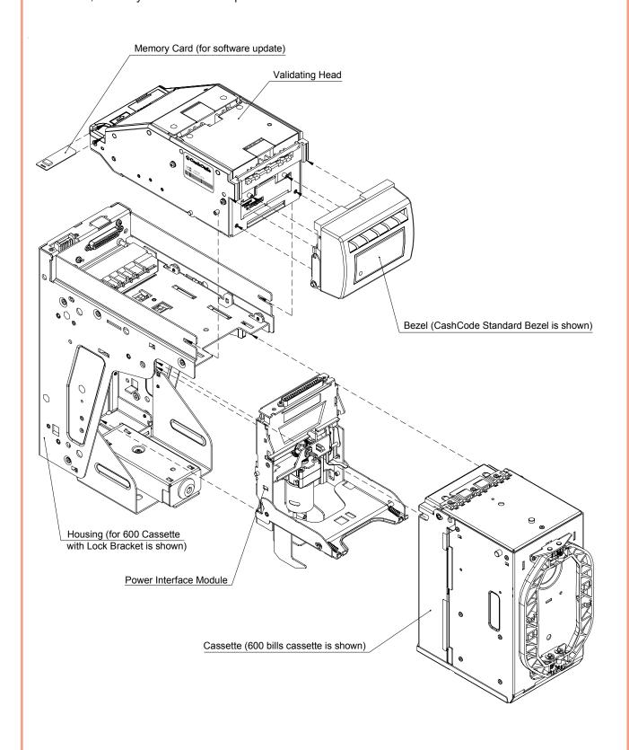
The FrontLoad bill validator is designed accommodate bills 62 to 82 mm wide and 125 to 172 mm llong – which encompasses most currencies.
