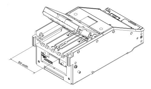
2) The Validating Head with a centering mechanism has a self-adjustable bill path. The width of the path is automatically adjusted to accommodate each bill. This type of Validating Head is used for currencies where the width of the bill changes with the denomination.
