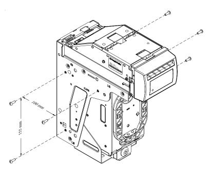
If the position of the mounting screws is different than the position of the mounting holes provided in the target equipment, then additional frame mounting components may be required.
