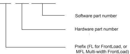
The Prefix defines the device class. Here FL means "FrontLoad Bill Validator" and MFL means "Multiwidth Front Load Bill Validator" (i.e. with a centering mechanism in the Validating Head).
