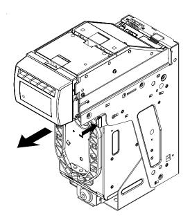
To replace the Cassette, close the Cassette cover, insert the Cassette into the FrontLoad frame, and turn the key to lock the Cassette back in place.
